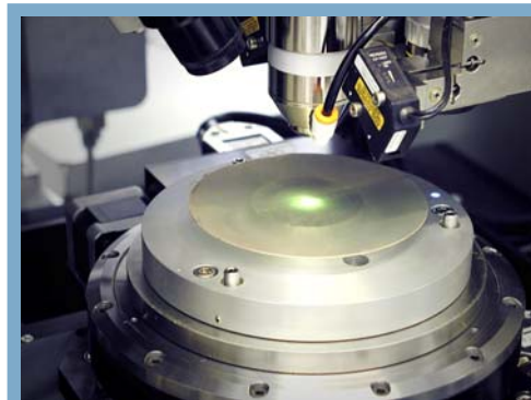
4 inch sapphire wafer scribing
